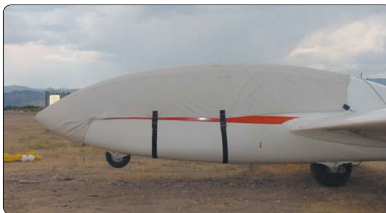
Figure 6-5. Protecting the canopy.
