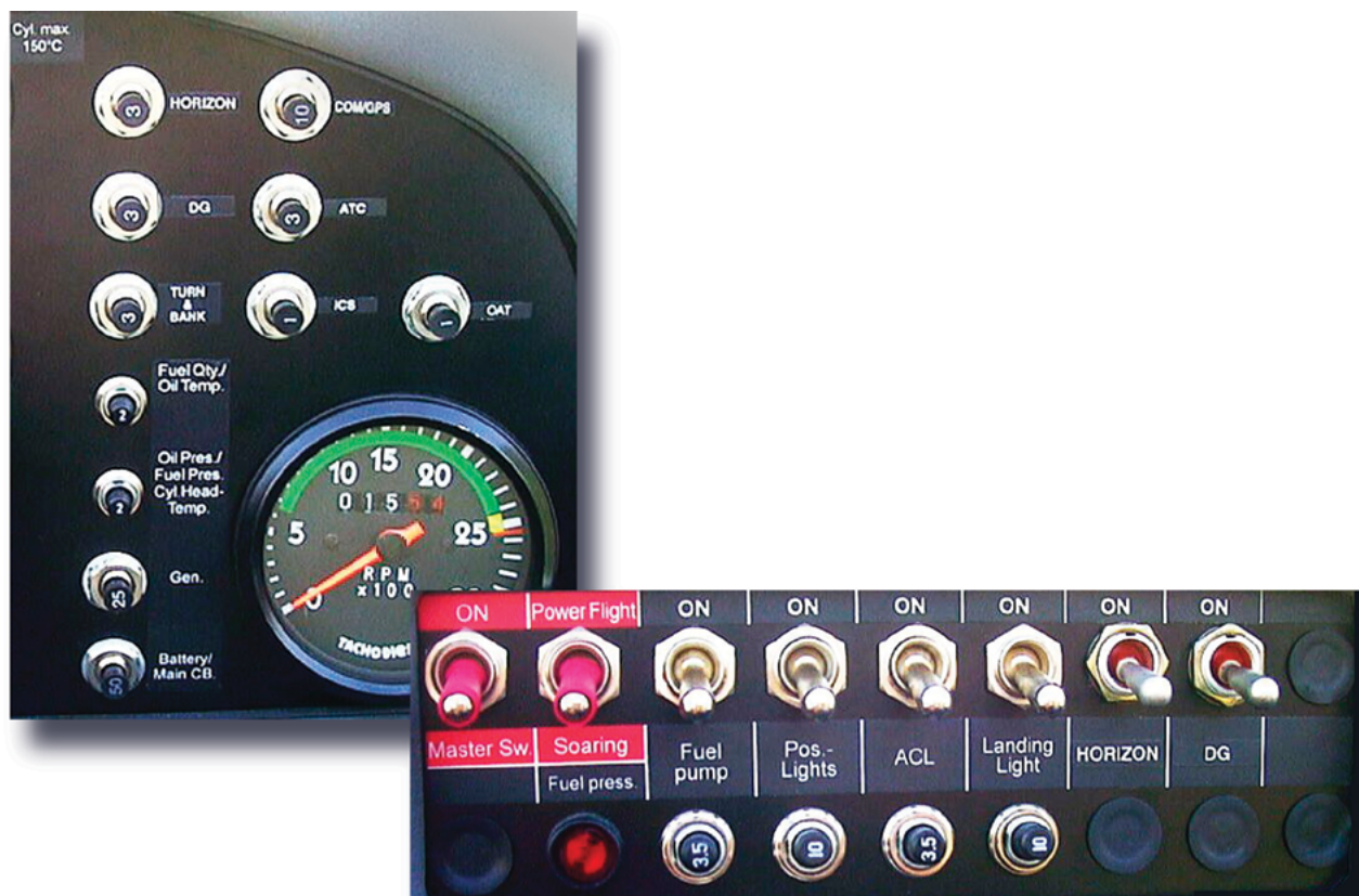
Figure 8-13. Self-launching glider circuit breakers.
