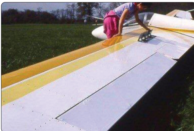
Figure 6-16. Positive control check of spoilers.
