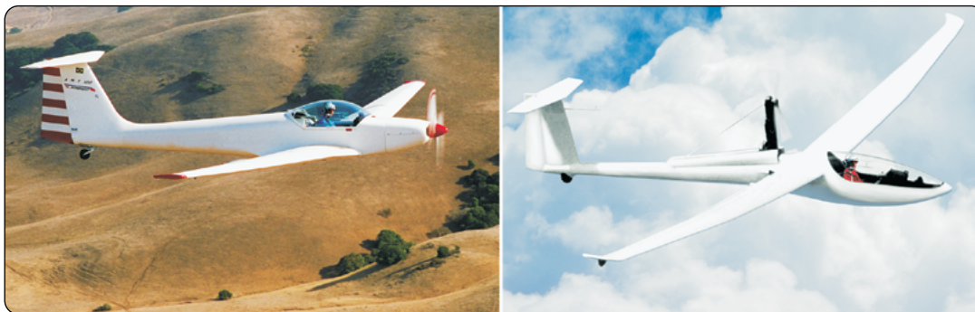
Figure 7-26. Types of self-launching gliders.
