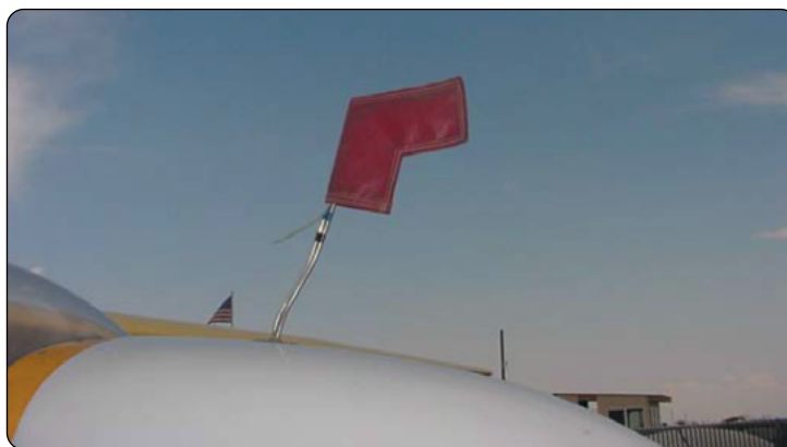
Figure 6-4. Protecting the pitot tube and total energy probe.
