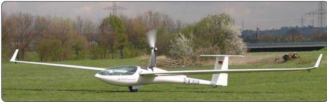
Figure 2-10. A DG-808B 18-meter high-performance glider in self-launch.
