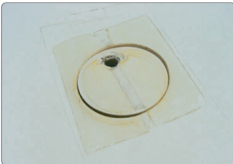
Figure 5-20. Water ballast tank vented filler cap.
