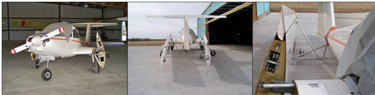
Figure 6-2. Folding the wings of the glider reduces storage space.
