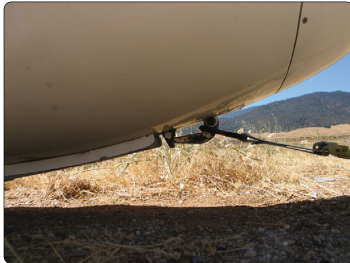
Figure 6-13. Schweizer-type tow hook.
