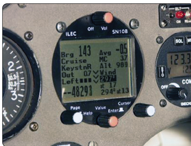
Figure 4-27. Glider flight computer display.
